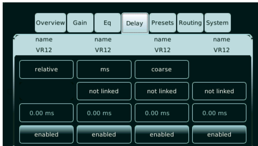
Fig 15. Delay tab, all channels enabled, delay “relative”
