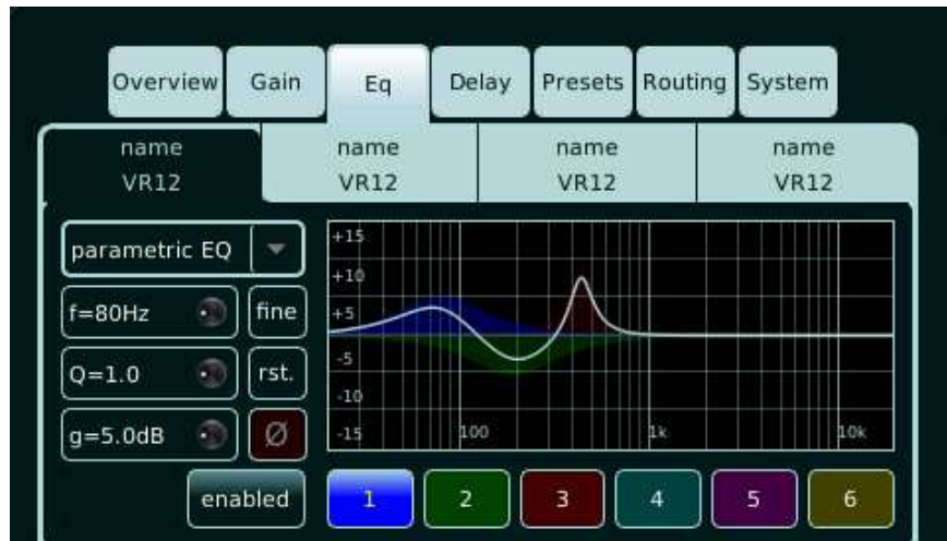
Fig 11. Equalizer section channel 1, band 1 parametric EQ enabled and active
