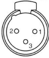
DMX - output XLR mounting-sockets (rear view):
