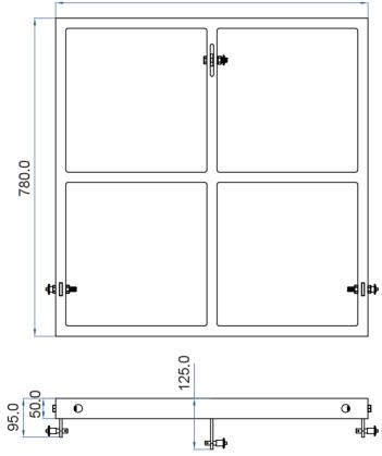
The WLA-28 WLA-28SUB fly frame is certified to hold a total weight(including third party hardware) of 450kg. Up to 12 WLA-28 and 1 WLA-28SUB elements can be flown with a safety factor of 12.
