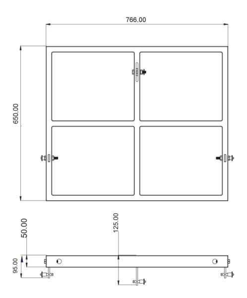
The WLA-28 Fly Frame is certified to hold a total weight (including third party hardware) of 450kg. 12 x WLA-28 and 1 x WLA-15B can be flown with a safety factor of 12.
