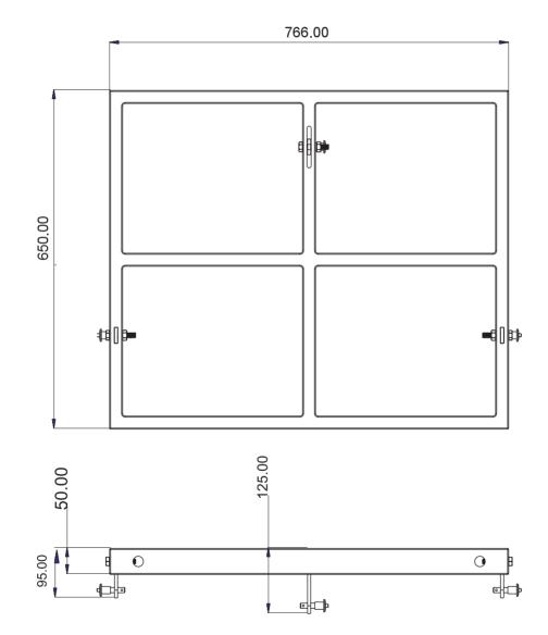
The WLA-28 Fly Frame is certified to hold a total weight (including third party hardware) of 450kg.  $12 \times WLA-28$  and  $1 \times WLA-15B$  can be flown with a safety factor of 12.
